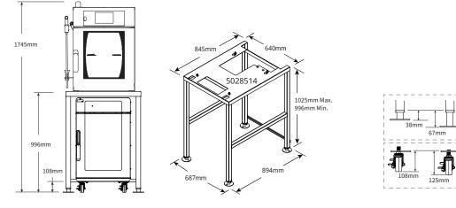
Dimensions shown are with adjustable feet and casters at minimum height.
