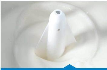
Tank Agitator. Prevents product stratification during storage and improves heat exchange during heat treatment.
