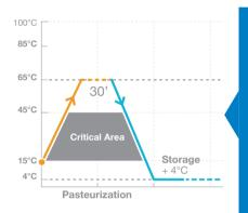
Optional Only for Super Tre AV EVO. With the automatic self-pasteurization system you can choose when to wash the machine up to a maximum interval of 42 days. As a further guarantee of hygienic safety, if the operator does not perform the complete cleaning at the end of the set days, the machine goes into automatic block.
