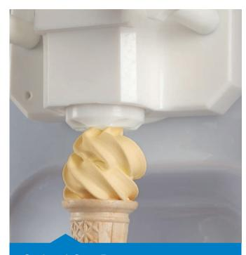
Optional Star Door. Allows the use of the new nozzles and the single-portion kit.
